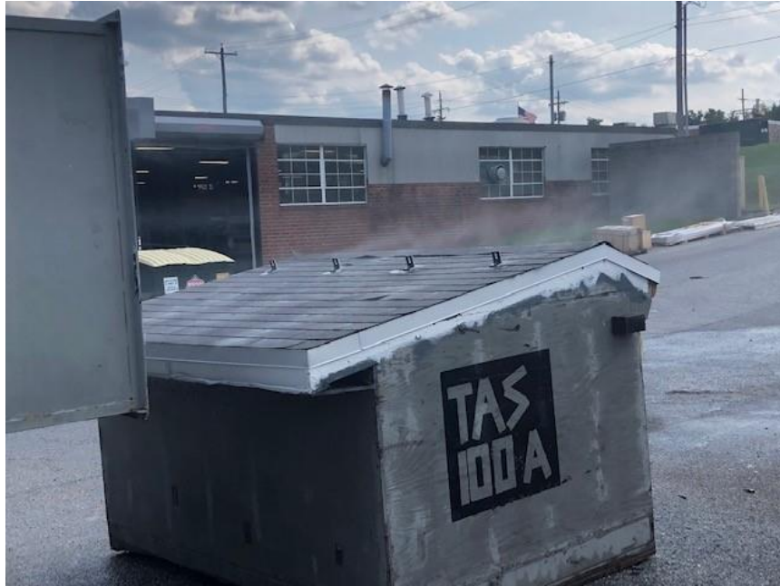
Photo No. 12 110 MPH Top Side
