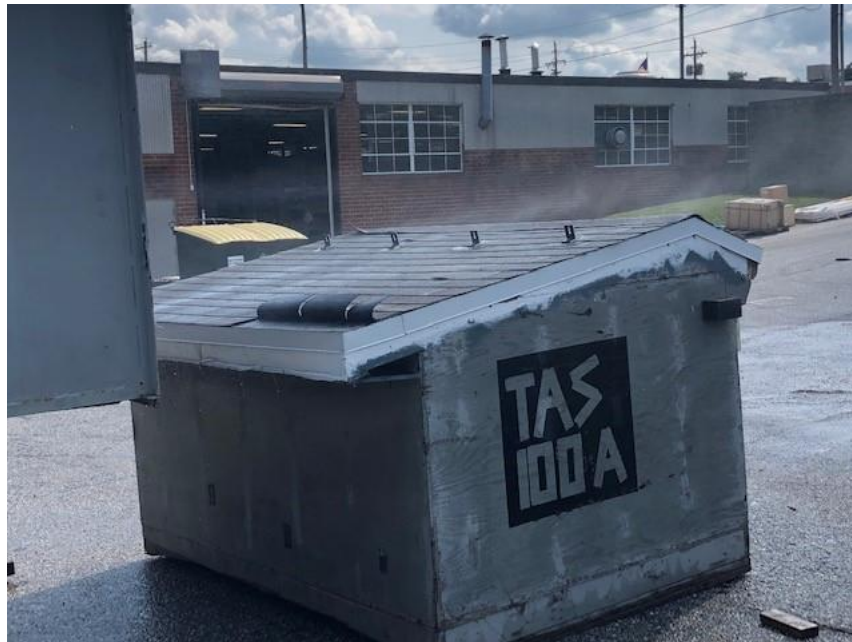
Photo No. 9 90 MPH Top Side
